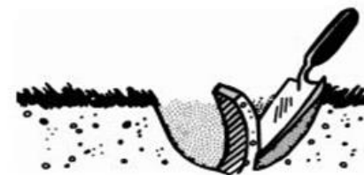
Figure 3. Soil sampling with a trowel.
