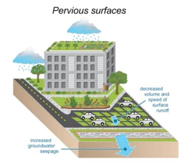
Image of a pervious surface -- "soft" surfaces like green roofs or rain gardens that decrease the volume of stormwater by soaking it into the surface medium.
