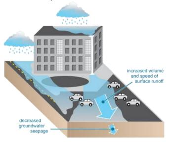
Image of Impervious Surfaces -- "hard" surfaces like roofs, roads, and parking lots that increase the volume of stormwater runoff.
