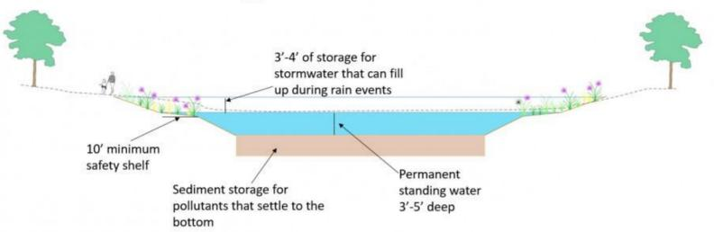
Engineers design these detention ponds using a formula for finding the volume of a cone. Ponds are not perfect spheres or rectangles, they start out wide at the top and get narrower the deeper you go. The formula for the volume of a cone is:
